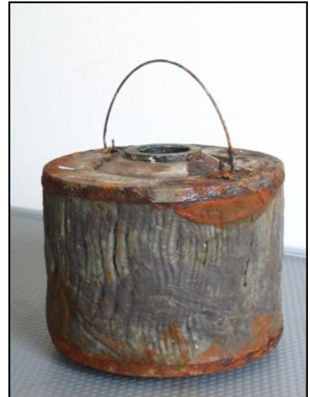
High soiled and slummed filter element
